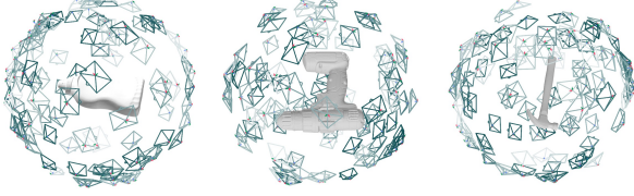
Fig. 6: Point completion Data Generation: Given the mesh/point cloud of the object, we render depth maps from 100 random views around a sphere of 1 unit looking at (0, 0, 0) , with the object in centered at the origin.
